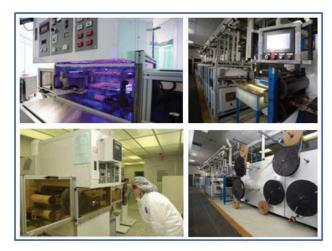
Interplex Etch Logic is a world-class supplier of chemically-etched metal components and a division of Interplex, a global contract manufacturer of complex components. The company's advanced "Chemical Stamping" process utilizes a highly consistent and highly repeatable reel-to-reel chemical metal etching process. More information can be found on the web at <a href="http://www.interplex.com/etchlogic">http://www.interplex.com/etchlogic</a>
